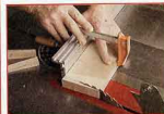
Clamp the blank to the miter gauge fence set at the correct angle and saw a wedge with a 3/32" blunt end. You need a second miter fence set to 90° to saw a second wedge.
