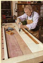
After gluing the backboard to the ends of the end caps, glue the plywood top tray into the groove in the backboard and screw and glue it to the underside of the benchtop.
