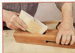
The next step is to check the fit of the wedge blank in your mortise.
