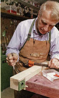
Bar clamps and hex-head bolts with captive nuts connect the end caps to the benchtop. Note the installation of the benchscrew nut in the short end cap.
