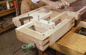
To assemble the tail vise, bolt the center guide rail to the fixed tail vise jaw and then bolt the outside guide block to the end cap. Finish up by installing the bench screw.
