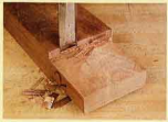
Slower is surer: knife the shoulder lines and clean up with a wide and sharp chisel.
