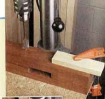
Use a 7/8" spade bit on center to leave a 1/16" of waste on each mortise wall.
