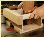
Clamp a rail square and upright in your tenoning jig. The jig guides the cut and keeps your hands safe during the operation.
