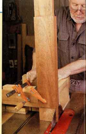
A block clamped in place on the front of the jig positions the rail to cut the cosmetic shoulder and avoids sawing into the jig.
